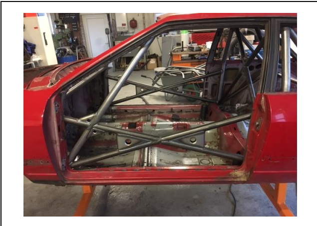
PHOTO 5 REAR BACKSTAY TO BODYSHELL ATTACHMENT
