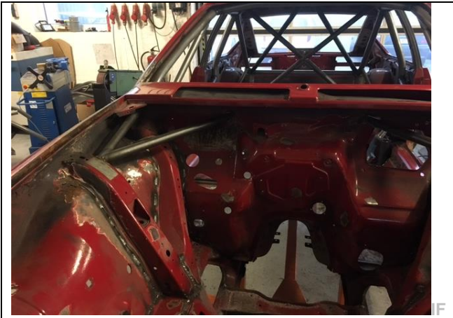
PHOTO 10 ANTI-INTRUSION DOORBAR - DRIVER
