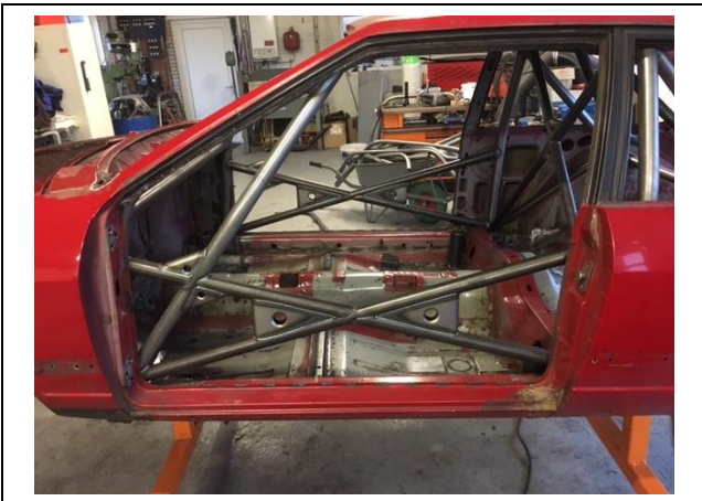
PHOTO 10 ANTI-INTRUSION DOORBAR - DRIVER
