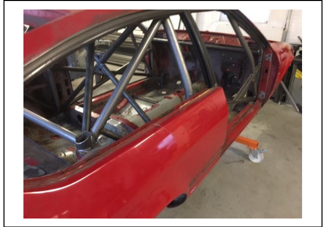
PHOTO 4 MAIN ROLLBAR TO FLOOR ATTACHMENT
