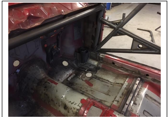
PHOTO 6 FRONT ROLLBAR TO FLOOR ATTACHMENT
