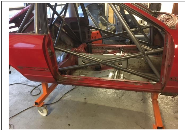
PHOTO 11 ANTI-INTRUSION DOORBAR - CO-DRIVER
