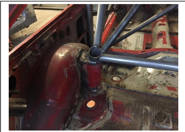
PHOTO 5 REAR BACKSTAY TO BODYSHELL ATTACHMENT
